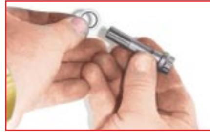
1. Clean and inspect all hardware for obvious damage. If necessary, chase or re-tap con rod threads to ensure proper thread engagement and accurate torque readings.
