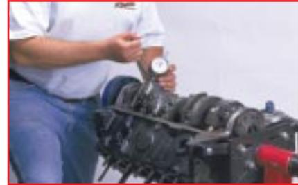
3. Assemble cap to rod, then lubricate with ARP Moly lube and install bolt & washer. Measure pre-torqued bolt length. You should keep a log of the original free standing length. A sample is on page 12.
