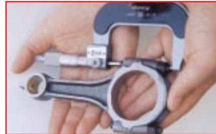
1. Inspect rods to ensure there is adequate chamfer to clear radius under heads, then install bolts after inspecting for damaged hardware.
