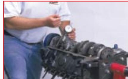
3. Lubricate rod nuts with ARP Moly lube, torque nuts to achieve recommended bolt stretch. A rod bolt stretch chart is located on page 13.
