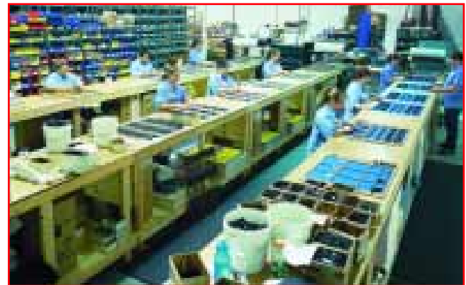
Components for each kit are placed on the appropriate display cards, sealed and labeled. Through-put has been significantly increased.
