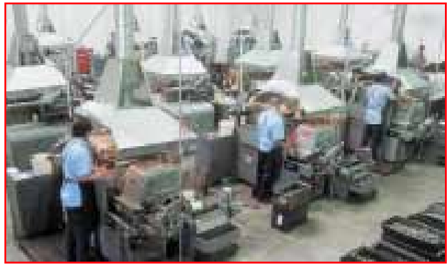
The Grinding Department is where all studs are centerless ground to ensure that they're perfectly concentric. As many as ten machining steps are required to achieve this level of accuracy.
