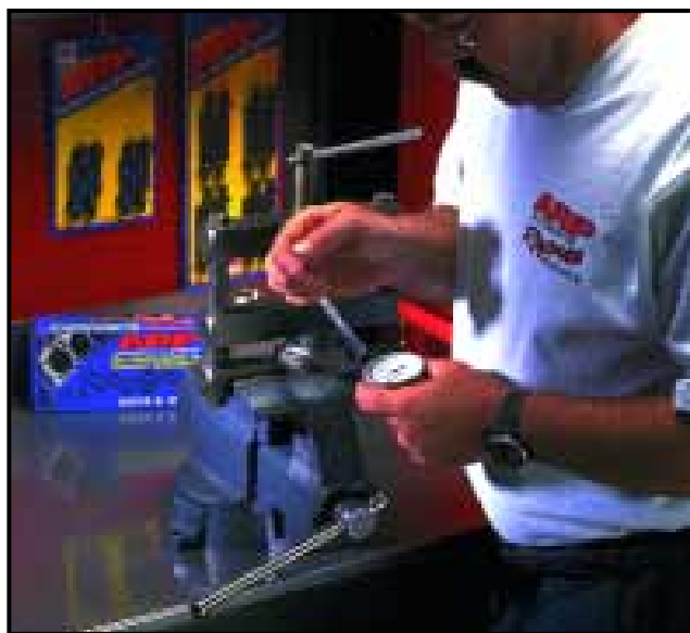
A rod bolt stretch gauge is one of the most important tools a serious engine builder can own. It's valuable in properly setting up a rod for resizing, obtaining the proper torque load when installed in the engine, and monitoring the condition of the bolt while in use.
