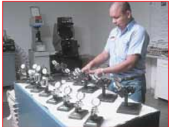
A series of special checking devices are employed to monitor the quality of threads. For every thread size, there's a checker.
