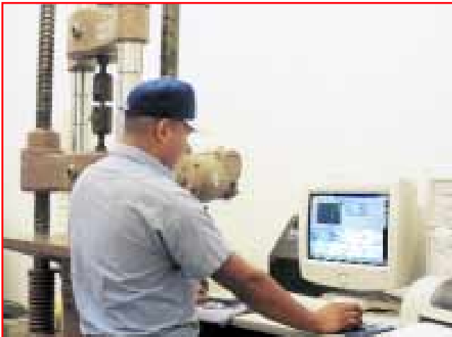
A computer-controlled Amsler Proof Loading device is used to determine the ultimate tensile strength of studs and bolts.
