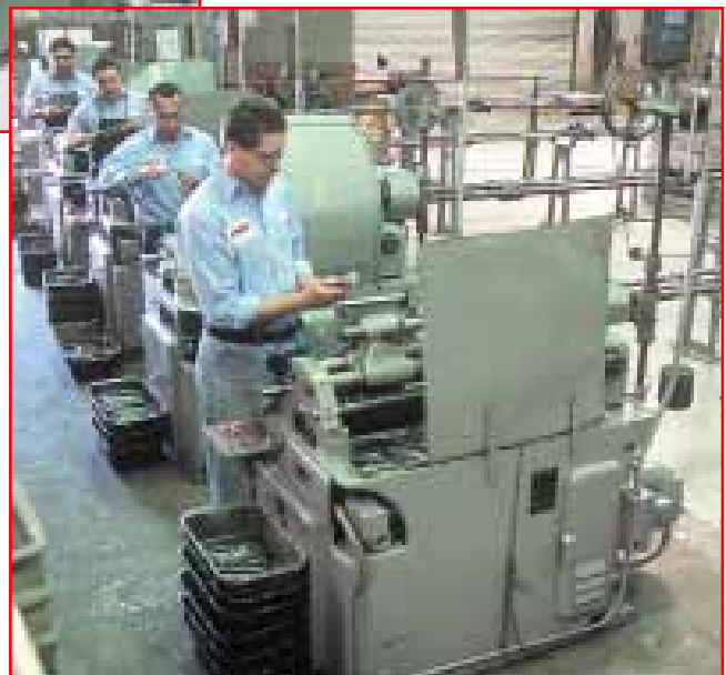
Here lengths of bar stock are automatically fed into special machines and cut to the appropriate length.
